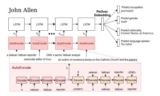
Figure 2: The model diagram: the main block is an LSTM, and the AutoEncoder is a module trained to learn to encode a sequence of words into a vector  $\underline{h}$ . Up to 10 introductions from one story are used to create an embedding; shown here are introductions for the Vatican analyst John Allen.
