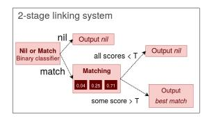
Figure 3: Two-stage stage linking system: Nil or Match followed by the Matching stage. This architecture helps improve accuracy at predicting *nil*.
